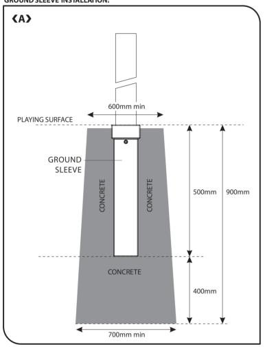
**NOTE:** Recommended foundation sizing only. Actual foundation depends on local ground conditions.
