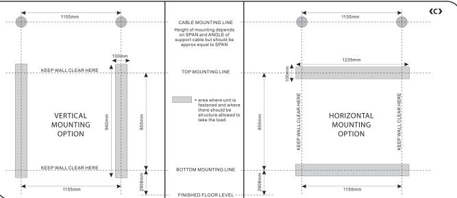
The unit can be mounted on a wall with **vertical** or **horizontal** supports as per diag <**C**> (specify on ordering).
