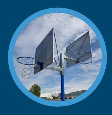
Backboards are HotShot steel  $1.2m \times 900$  perforated to reduce wind resistance and weight, electro galvanised and powder coated finish. Plywood, stainless steel, and glass backboards are also available in the same dimentions.
